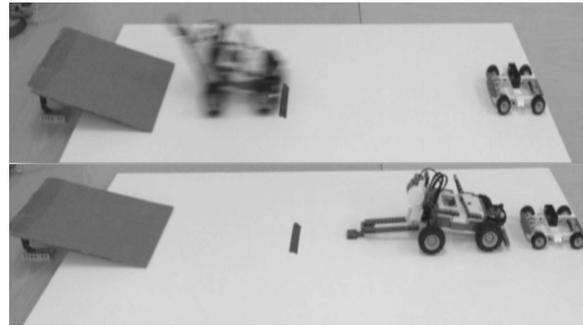
Fig. 1. A SLIDER truck engages its auto-sensing emergency brake to avoid a collision.
